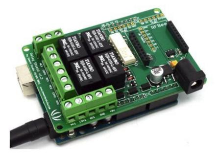
Step1. Plug Relay Shield onto Arduino Duemilanove (or compatible) board;
