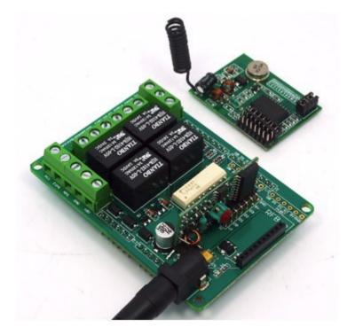
Step1. Plug and solder the Receiver onto the Relay Shield.
