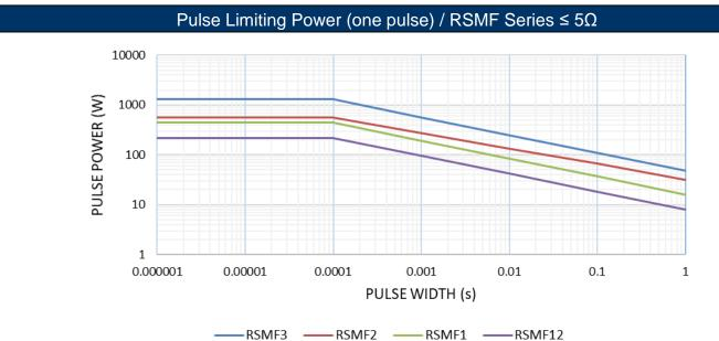
Pulse Limiting Power (one pulse) / RSMF Series  $\geq 5\Omega$
