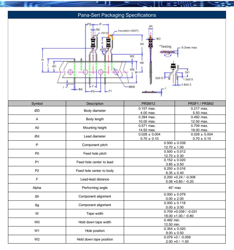
General Purpose Metal Oxide Resistor
