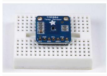
Position the Breakout Place the breakout board over the short end of the header pins.
