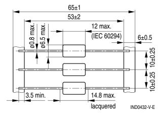
Dimensions in mm Minimum lead spacing 15 mm
