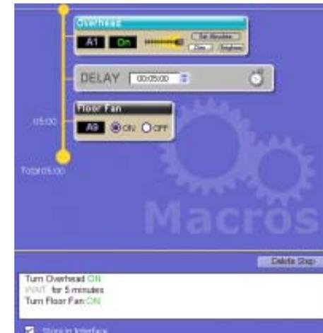
Lamp modules and other dimmable modules have several options. To turn a module On, simply select "Set Absolute" and adjust the level to On (all the way to the right). Off works the same way.
