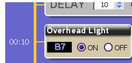
If you add a lamp module or other dimmable module to your macro, you have two different options. If you use “Set to” ActiveHome Pro will turn your module on to full brightness, then dim it to the selected level. If you use “Adjust by” ActiveHome Pro will just tell your module to dim or brighten, which only works if the module is already on.
