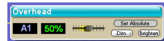
The “Dim” and “Brighten” settings work differently. If you have a module that’s already on, use “Dim” or “Brighten” to tell it to dim or brighten by a certain amount. Use the slider to select the amount you want to the light to change.
