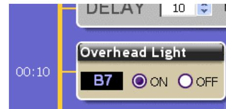
If you add a lamp module or other dimmable module to your macro, you have two different options. If you use “Set to” ActiveHome Pro will turn your module on to full brightness, then dim it to the selected level. If you use “Adjust by” ActiveHome Pro will just tell your module to dim or brighten, which only works if the module is already on.
