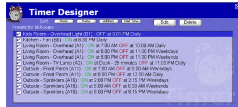
In the Summary View you can check or uncheck timers to turn them on or off, and delete timers as well. Use the **Room**, **Module**, **Address**, and **Start Time** buttons to change the sort order of the timer listing.
