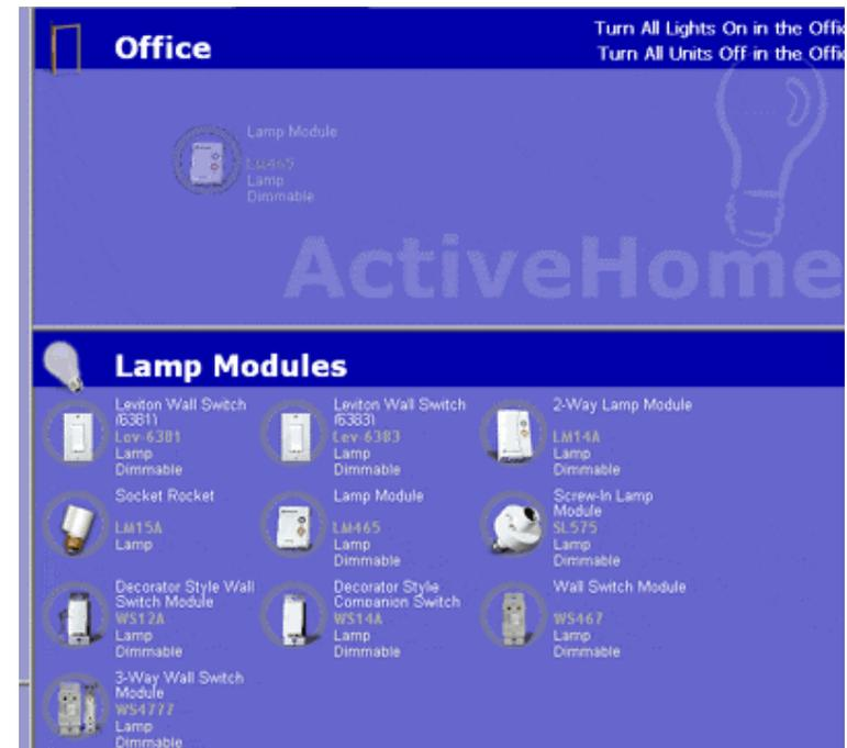
When you drop the module, all the important information is filled in automatically. If you want to change the name of the module or its address, click into the module and enter the new information.
