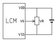
$V_{DD}$ -V<sub>0</sub>: LCD Driving voltage VR: 10k~20k
