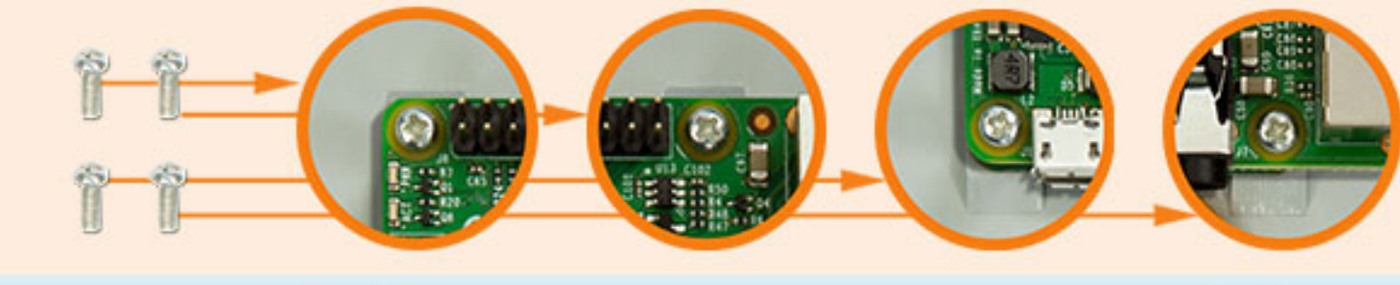
Use the 4 x screws to secure the Raspberry Pi board to the Standoffs then connect the DSI ribbon cable to the Raspberry Pi
