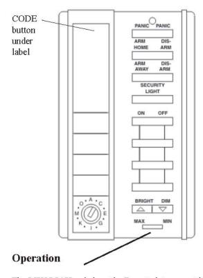
The MIN/MAX switch on the Remote lets you set it to arm the system with or without an exit/entry delay.
