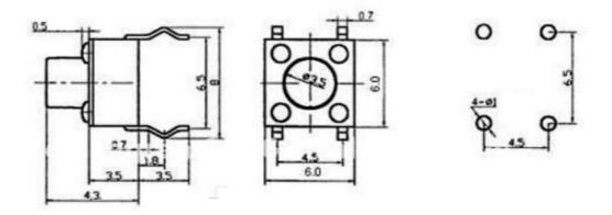
Terminal Arrangement/Internal Connections (Top View)
