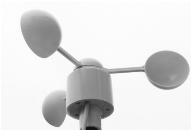
Figure 9.20 A cup anemometer for measuring wind speed.
